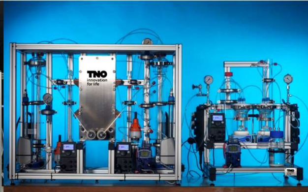
Flow cell electrolyzer continuous bench scale system
