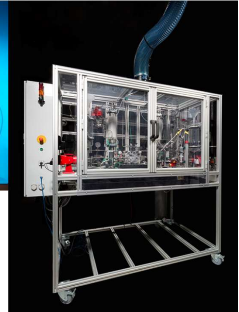
Flow cell electrolyzer continuous autonomous bench scale system
