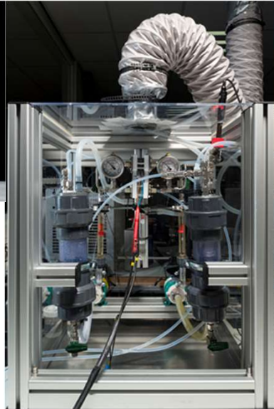
Flow cell electrolyzer batch bench scale system
