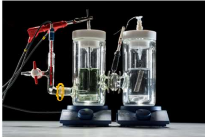
Electrolysis conditions: glass electrolysis cell
